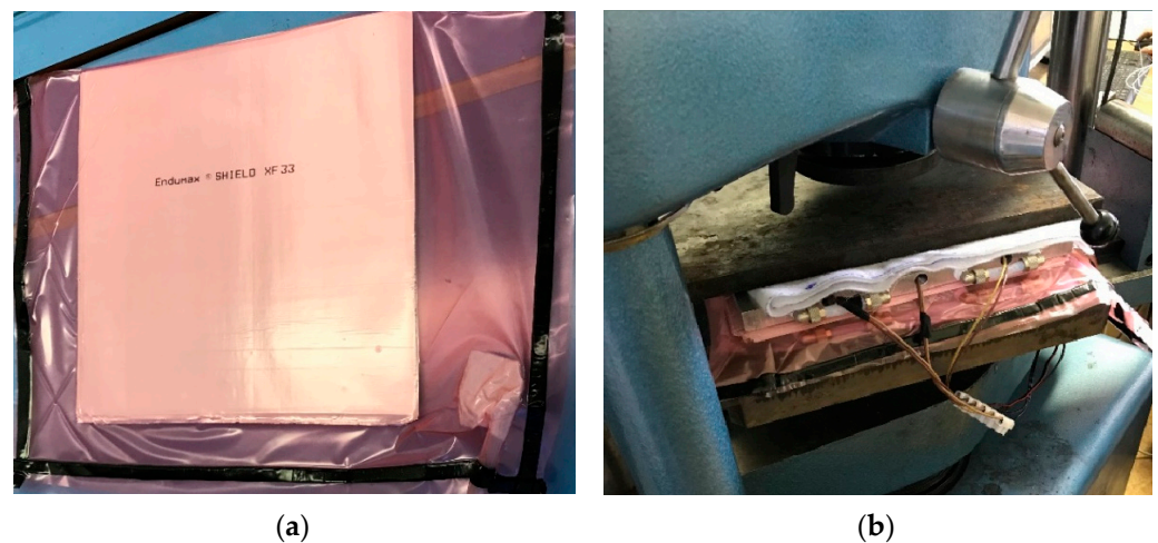
Figure 5. Manufacture of composite panels by hot-pressing technology: (a) material preparation Endumax Shield XF33; (b) hydraulic press ZD40.
