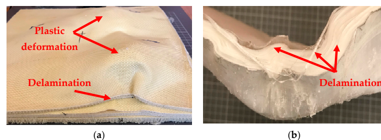
Figure 16. Deformation and delamination of composite panels: (a) Twaron CT 747, ER68; (b) Endumax Shield XF33.
