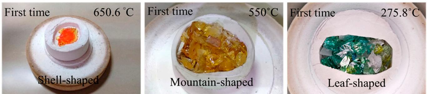
**Figure 4.** Results of the first cast glass trial firing.
