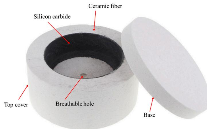
**Figure 1.** Schematic diagram of the microwave kiln.
