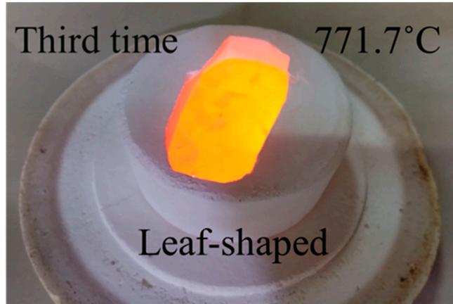
**Figure 6.** Results of the third cast glass trial firing.
