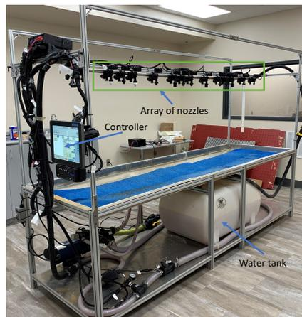
**Figure 1.** Experimental setup with crop spray nozzles for droplet data collection.
