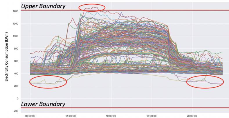
**Figure 1.** An example to illustrate the problem of the “IQR” method. The red circled parts highlight the “False Positive” outliers detected by the upper boundary and the “False Negative” outliers not detected by the lower boundary.
