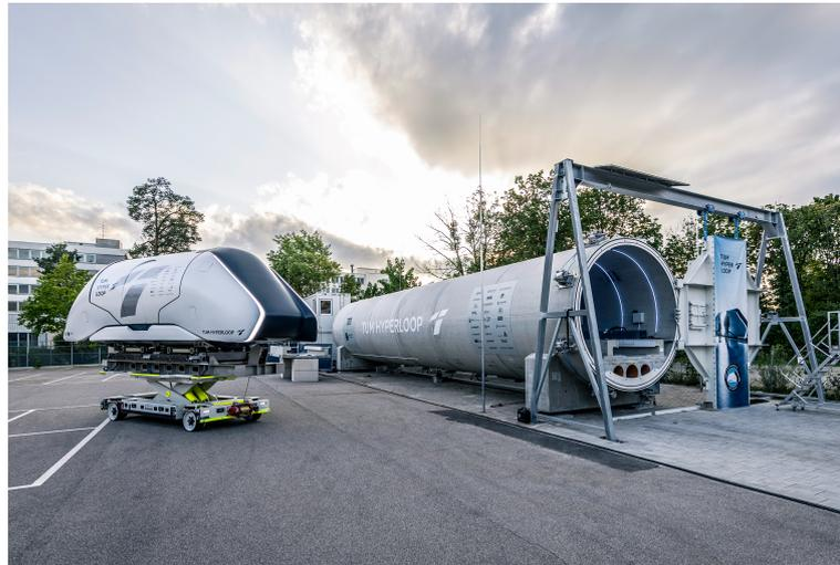
**Figure 1.** Photo of the TUM Hyperloop Demonstrator. On the left, the pod, with a capacity for five passengers, is shown, standing on a separate vehicle to be transported from the workshop to the tube. On the right, the 24 m long tube, with a diameter of 4.2 m, can be seen. The concrete tube can be sealed to be vacuum-tight by a steel door.
