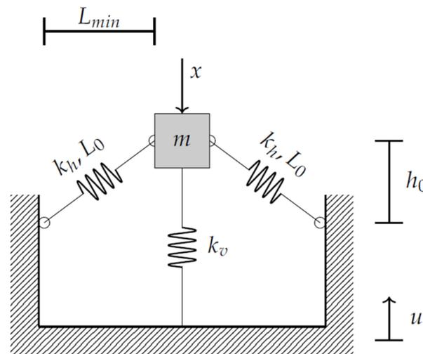
Figure 3. Negative stiffness oblique spring mechanism.
