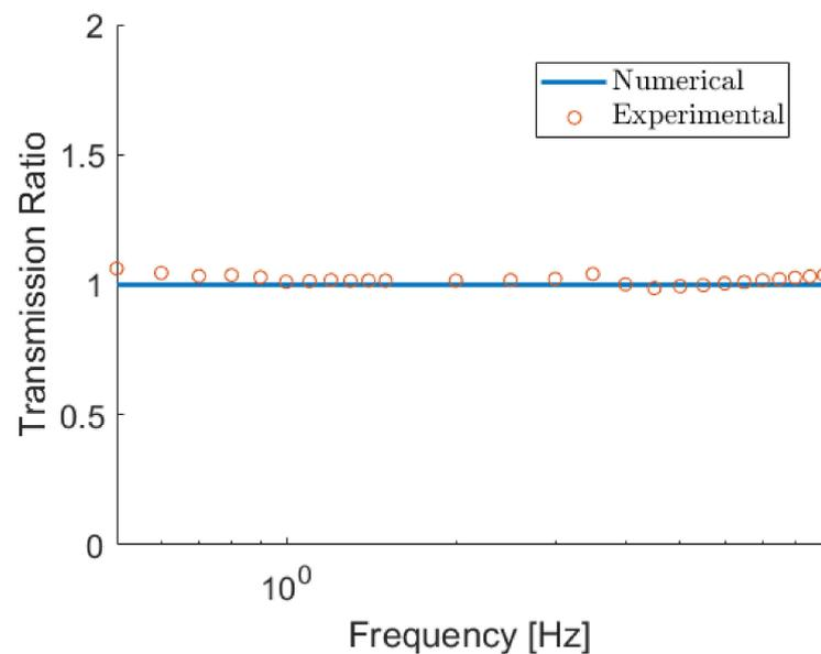
**Figure 16.** Mass 2 transmissibility within the universal seat in combination with the quasi-zero stiffness (QZS) cushion.
