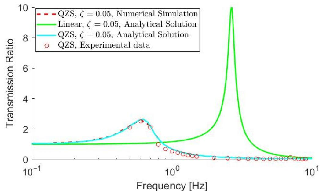
**Figure 11.** Comparison of the experimental, analytical, and numerical results for the quasi-zero stiffness (QZS) cushion. The analytical response of a similar linear system is included for reference. For all plots, the mass, vertical stiffness, and damping are identical. In the case of the QZS system, tuned oblique springs are added.
