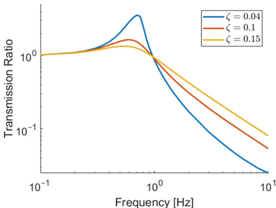
**Figure 14.** Effect of increasing viscous damping ( $\zeta$ ) within quasi-zero stiffness cushion.
