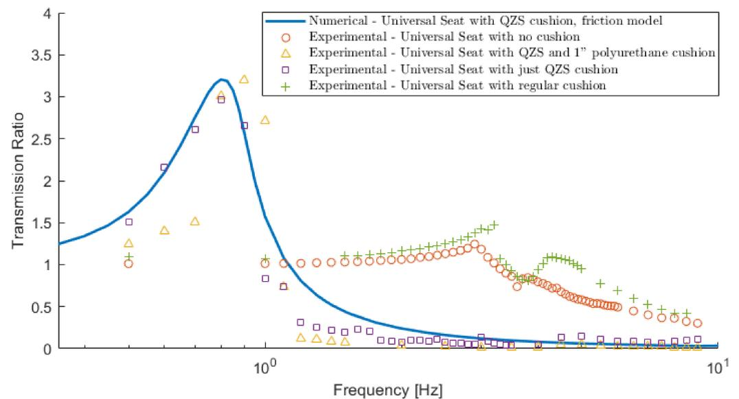
**Figure 12.** The response of the overall universal seat with a regular cushion and the quasi-zero stiffness (QZS) cushion.
