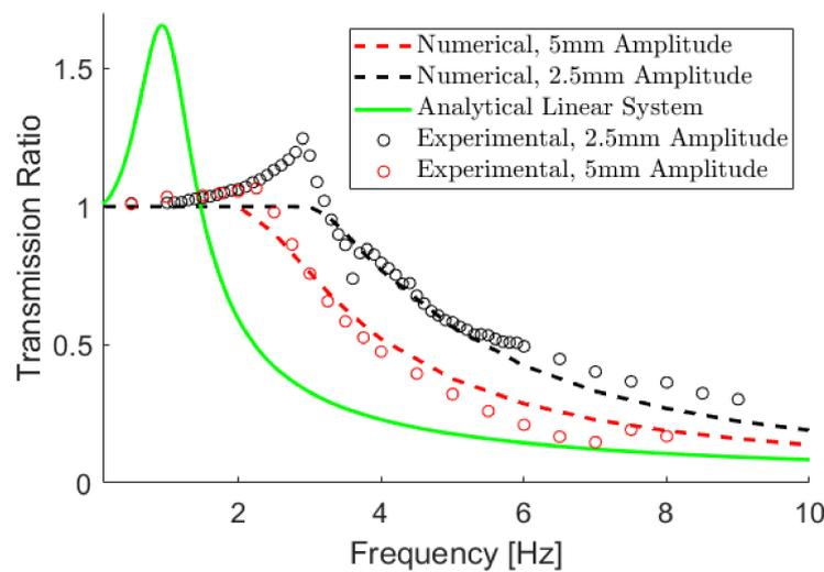
**Figure 9.** The experimental dynamic response of the universal tractor seat compared to the expected linear response and the numerical simulation with the Force Balance Friction Model. In all cases,  $m = 81.9 \text{ kg}$ ,  $\zeta = 0.4$ ,  $k = 3420 \text{ m/N}$ , and  $v_o = 0.001 \text{ m/s}$ .
