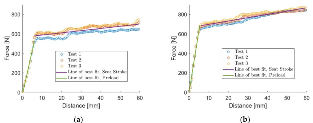
**Figure 6.** A force–displacement plot of the universal tractor seat as a single-degree-of-freedom system. (a) The Instron applies its force near the front of the seat; (b) the Instron applies its force near the back of the seat. In each plot, the green line is fit to the preload portion of the plot and the purple line to the main stroke of the seat. When a mass is placed on the seat, the seat vibrates entirely within the “Seat Stroke” region.
