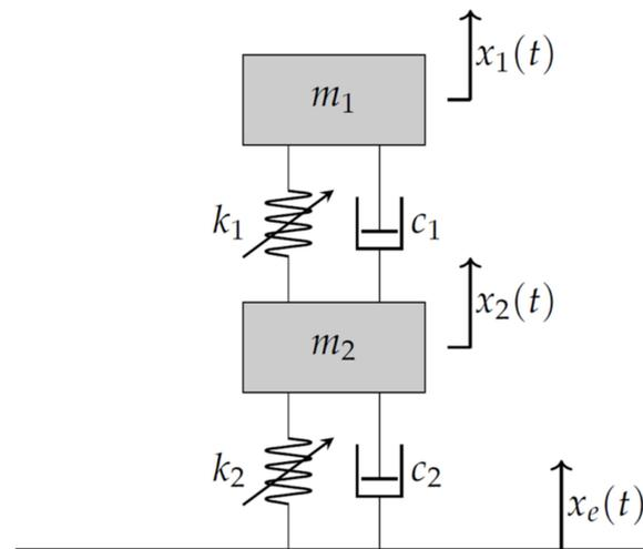
**Figure 1.** The model of a two-degree-of-freedom system consisting of nonlinear stiffness elements.
