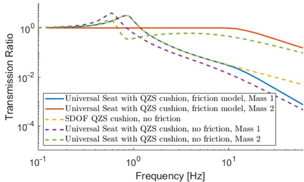
**Figure 15.** Theoretical response of universal seat and quasi-zero stiffness (QZS) cushion with and without friction.
