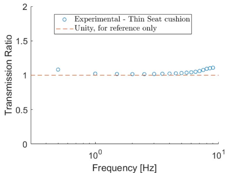
**Figure 13.** Dynamic response of the one-inch polyurethane foam pad used on the quasi-zero stiffness (QZS) cushion between 0.5 and 9 Hz.
