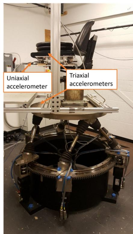
**Figure 4.** Overall experimental setup of universal tractor seat with quasi-zero stiffness cushion on top.
