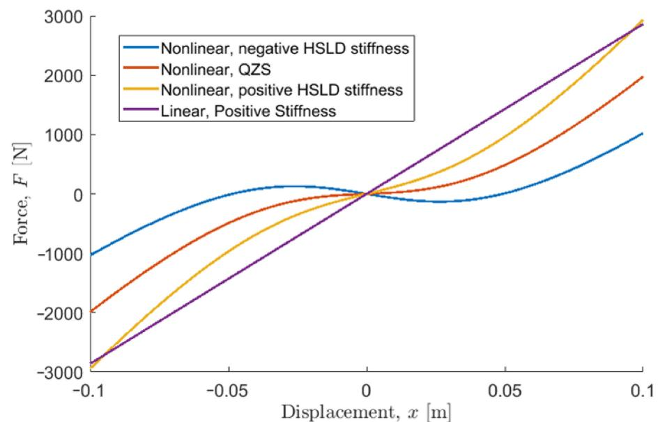
**Figure 2.** The stiffness of a High-Static Low-Dynamic (HSLD) system when tuned to have localized positive, negative, and quasi-zero stiffness (QZS).
