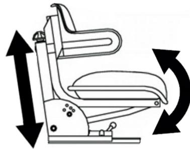
**Figure 7.** Diagram of stock universal tractor seat, containing two potential degrees of freedom.
