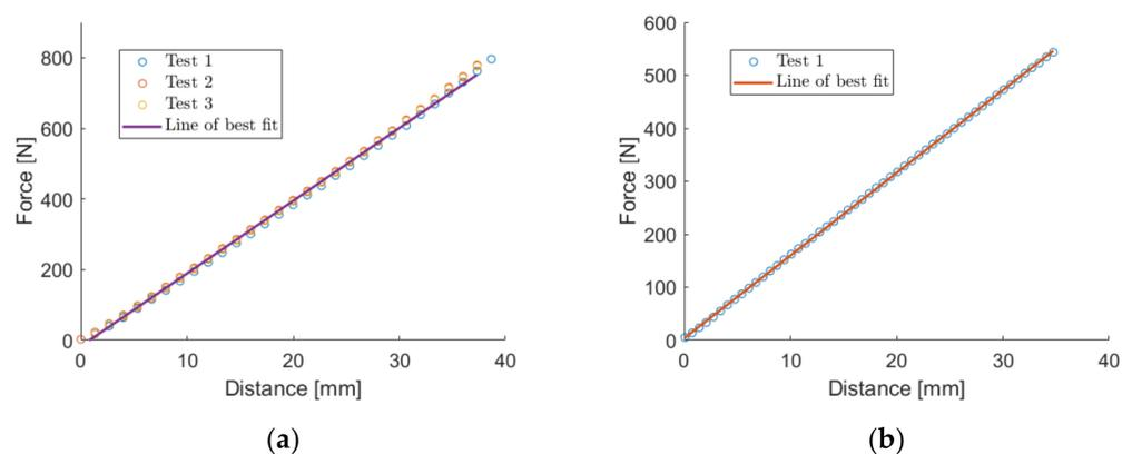
**Figure 8.** Spring stiffness of springs within quasi-zero stiffness cushion. (a) Spring stiffness of vertical springs approximated by line of best fit; (b) Spring stiffness of ten oblique springs in parallel approximated by line of best fit.
