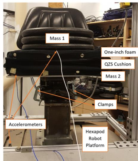
**Figure 10.** Universal tractor seat with quasi-zero stiffness and foam cushion on top of it.
