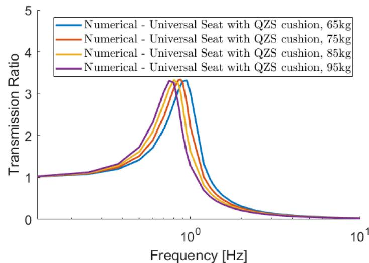
**Figure 17.** The effects of changing mass on the universal seat with the quasi-zero stiffness (QZS) cushion, assuming that the cushion is tuned to the point of lowest stiffness.
