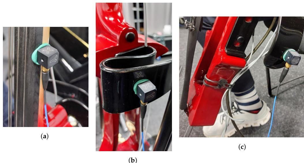
**Figure 3.** Accelerometer attached at various locations on the haptic cello, each corresponding to those on the acoustic instrument. (a) Neck: left-hand grip (for right-handed players). (b) Top back: chest contact. (c) Side: inner thigh contact.
