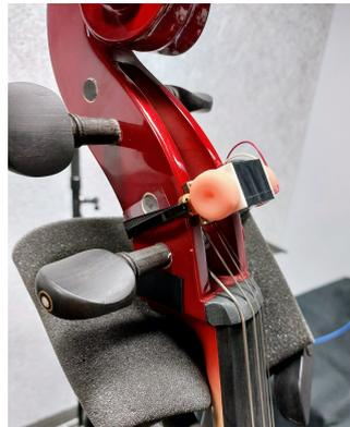
**Figure 1.** A Tactile Labs Haptuator BM3C vibrotactile transducer attached to the scroll of the instrument.
