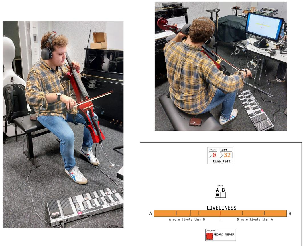
**Figure 4.** The experimental setting, and a close-up of the GUI for rating the qualitative attribute *liveliness*.
