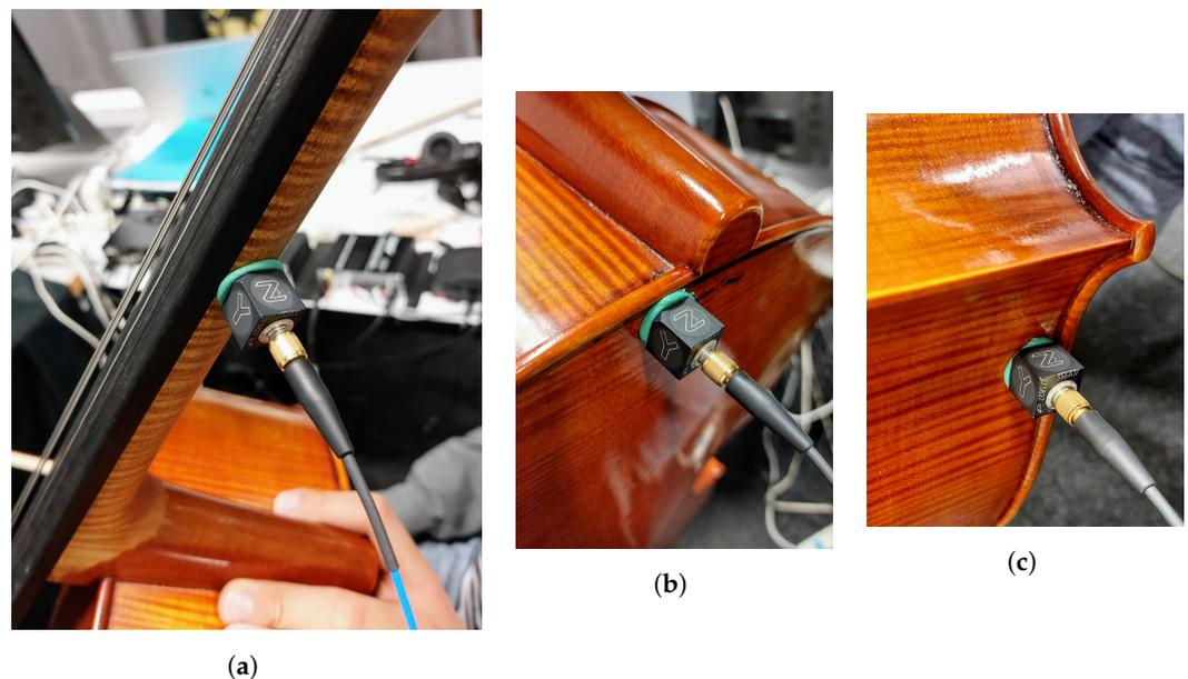
**Figure 2.** Accelerometer attached at various locations on the acoustic cello, each typically in contact with the player’s body. (a) Neck: left-hand grip (for right-handed players). (b) Top back: chest contact. (c) Side: inner thigh contact.
