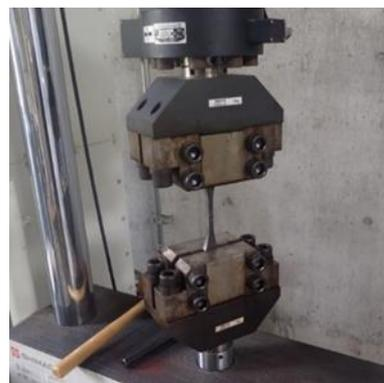
Figure 14. Photo of fatigue test.
