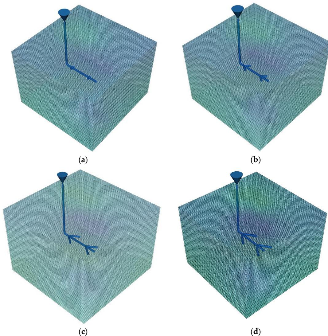
**Figure 5.** Comparative illustration of fishbone wells with varying lengths of branches: (a): 150 m, (b): 300 m, (c): 450 m, and (d): 600 m.
