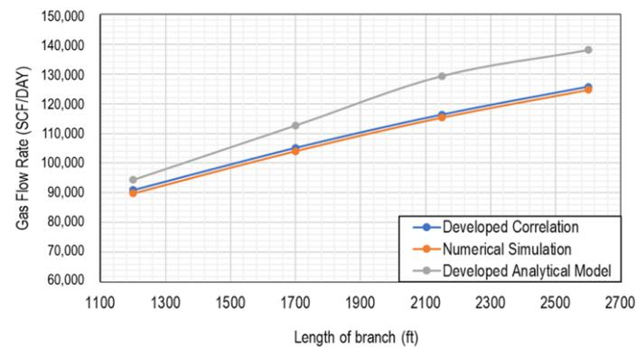
**Figure 6.** The effect of the length of branches on the cumulative production (Ouardi et al. [13]).
