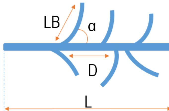
**Figure 2.** Fishbone well design, LB: length of the branch,  $\alpha$ : angle between branch and main lateral, D: distance between branches, L: length of the main lateral of the fishbone [15].
