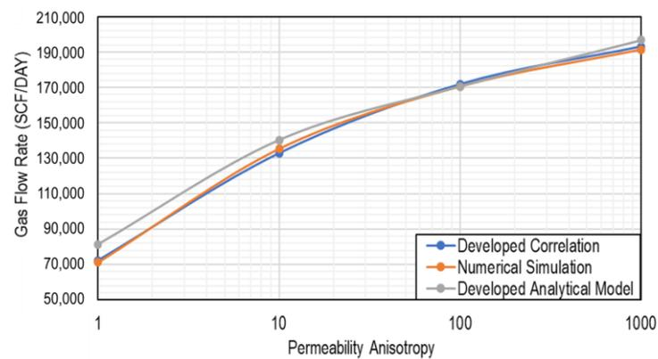
**Figure 8.** The effect of permeability anisotropy on cumulative production (Ouadi et al. [13]).
