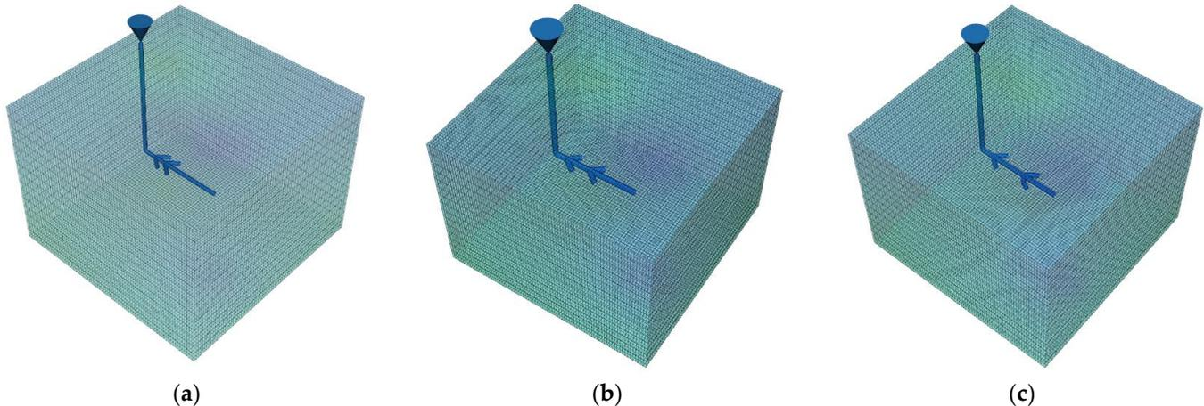
**Figure 9.** Comparative illustration of fishbone wells with distance between branches: (a): 100 m, (b): 200 m, and (c): 300 m.
