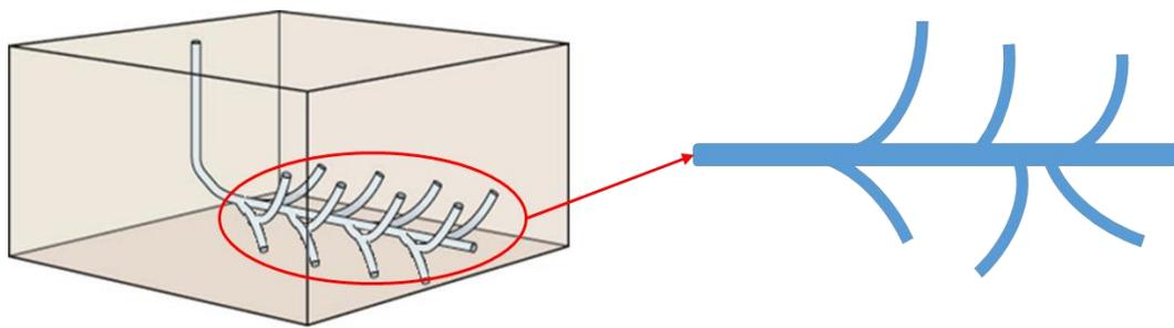
**Figure 1.** Fishbone drilling technology [5].
