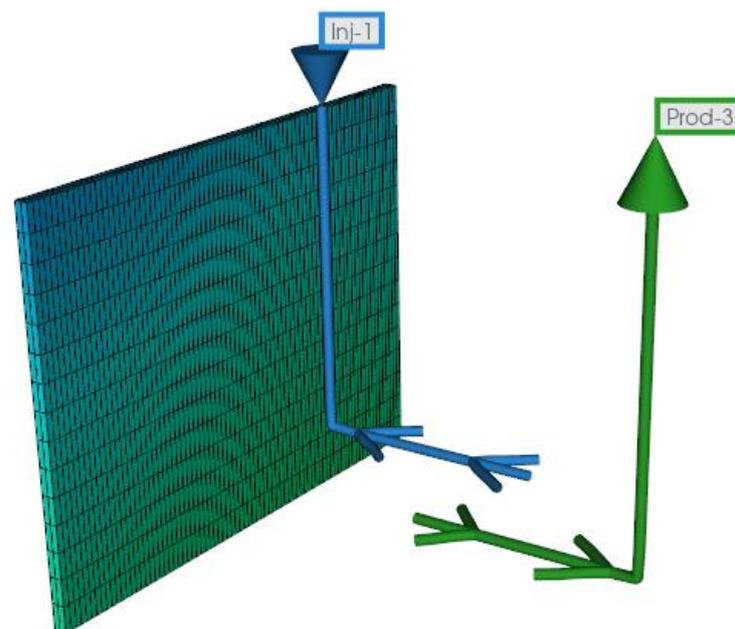
**Figure 13.** Advanced representation of fishbone well structures within a reservoir model.
