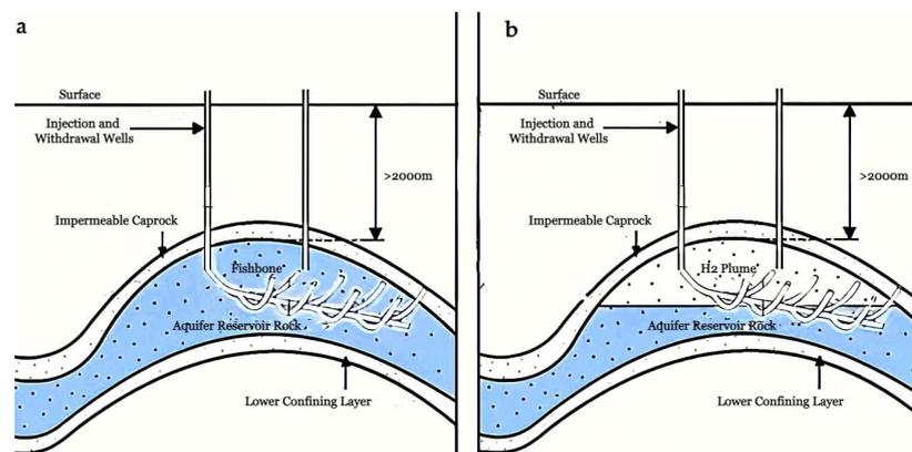
**Figure 12.** Fishbone for hydrogen storage in saline aquifers. (a) before injection, (b) post injection.
