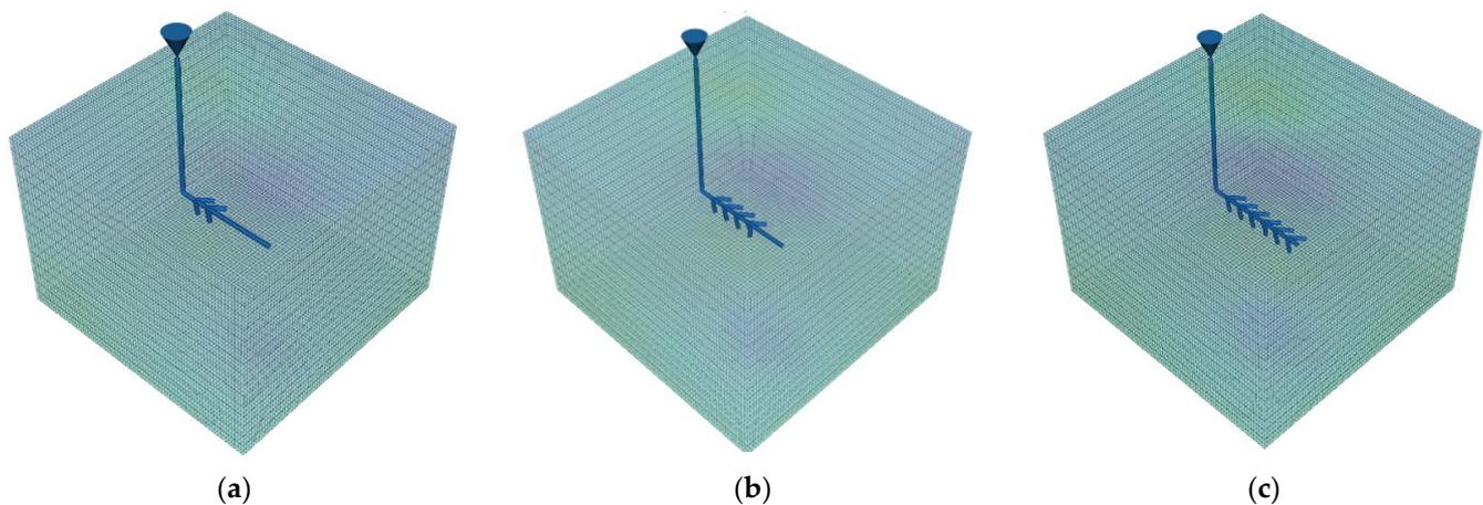
**Figure 3.** Comparative illustration of fishbone wells with varying branch numbers: (a): 4 branches, (b): 8 branches, and (c): 16 branches.
