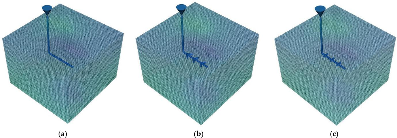
**Figure 7.** Comparative illustration of fishbone wells with varying angles between the branch and the main lateral: (a):  $20^\circ$ , (b):  $45^\circ$ , and (c):  $90^\circ$ .
