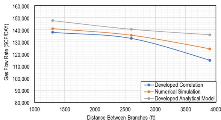
**Figure 10.** The effect of the distance between adjacent branches on the cumulative production (Ouadi et al. [13]).
