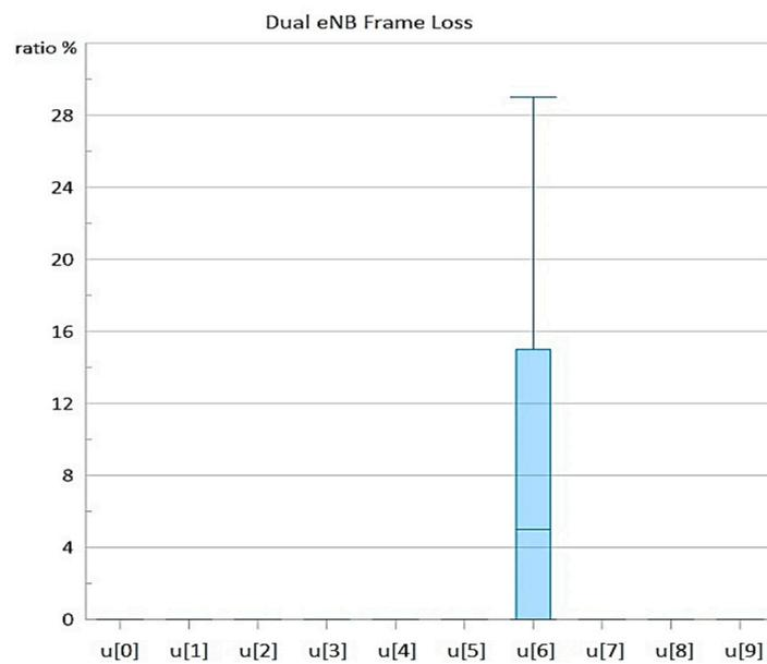
Figure 7. UEs’ simulated frame loss (Dual eNB).
