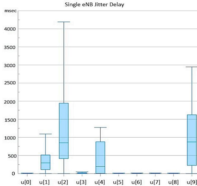
**Figure 8.** UEs’ simulated jitter delay (single eNB).
