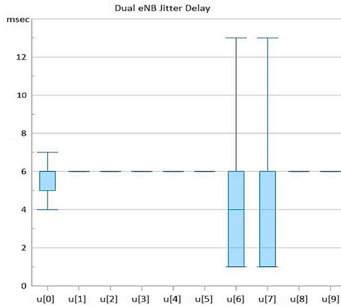
Figure 9. UEs’ simulated jitter delay (dual eNB).
