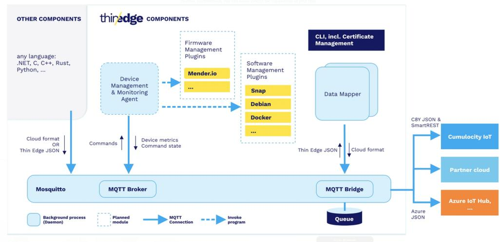
Figure 12. Thin-edge.io architecture [67].
