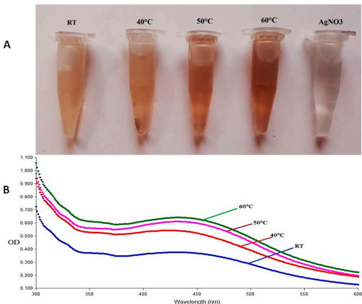
**Figure 2.** (A) AgNPs synthesized using bacteria at different temperatures. (B) UV-vis absorption spectra of AgNPs synthesized by soil bacteria at different temperatures.
