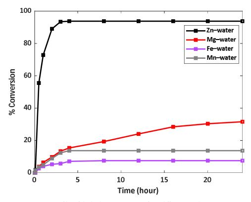
Figure 2. Kinetic profiles of the hydrogen generation from different metal-water systems at 60 °C.
