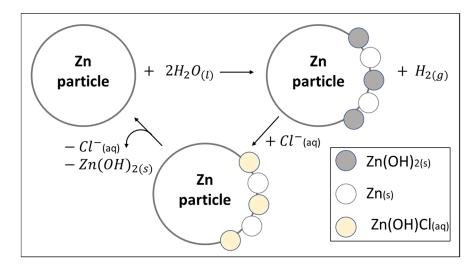
Figure 5. Cleaning process of zinc surface by chloride anion.
