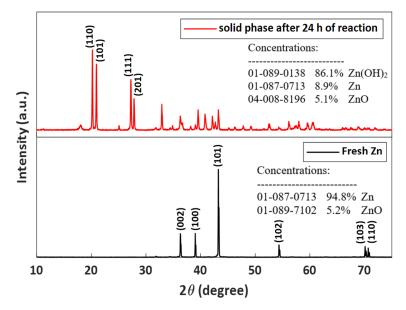
Figure 3. PXRD patterns of fresh zinc before reaction (black) and of the reaction mixture after 24 h of reaction (red).
