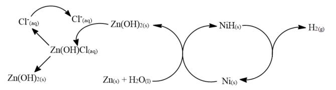
**Figure 7.** Catalytic mechanism of hydrogen generation from zinc–water system that is catalyzed by nickel nanoparticles formed in situ.
