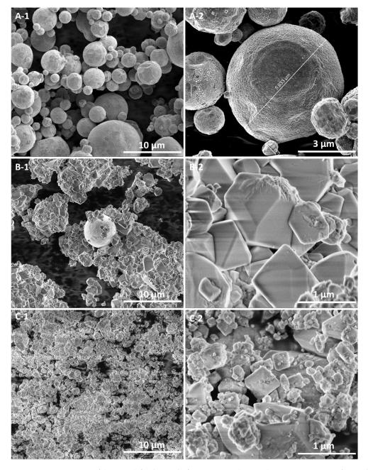
**Figure 4.** SEM images of (**A-1**,**A-2**) fresh zinc before reaction, (**B-1**,**B-2**) reaction mixture after 12 h of reaction, and (**C-1**,**C-2**) reaction mixture after 24 h of reaction.
