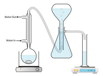
Figure 1. The flow-meter setup for monitoring the volume of hydrogen release.
