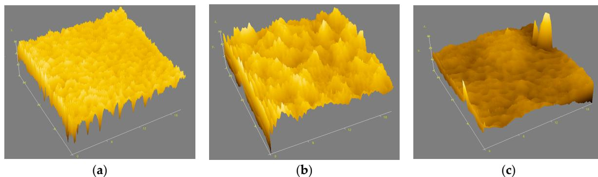
**Figure 4.** AFM image of the film surfaces: (a) PA; (b) PB; (c) PC.
