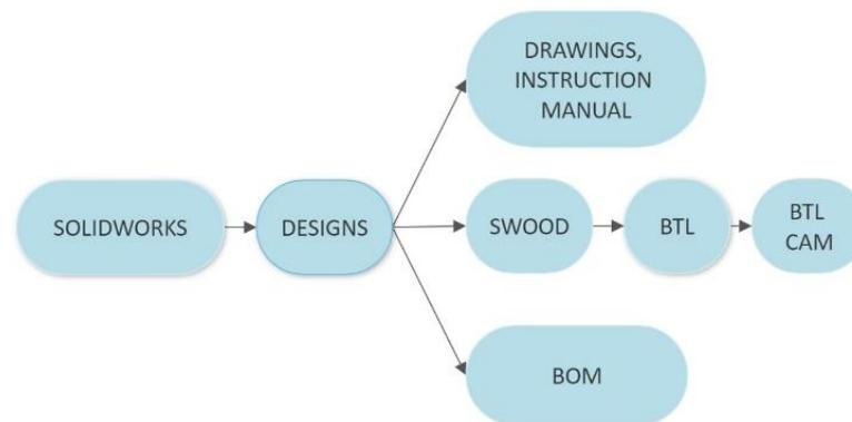
**Figure 1.** Process pipeline.
