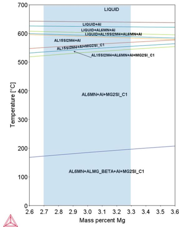
Figure 3. Pseudo—binary phase diagram for 5754 alloy composition.
