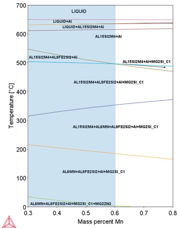
Figure 4. Pseudo—binary phase diagram for 3105 alloy composition.
