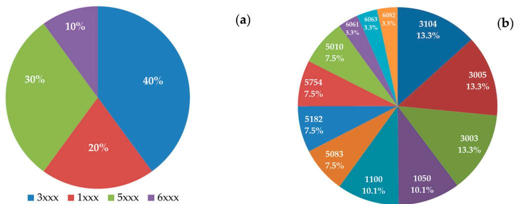
**Figure 1.** (a) Graph showing the consistency of aluminum, (b) Graph showing the percentage of each aluminum alloy in the scrap.
