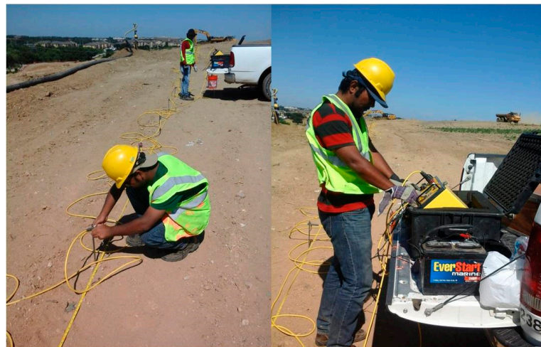
Figure 6. The authors conducting resistivity tomography at the site.
