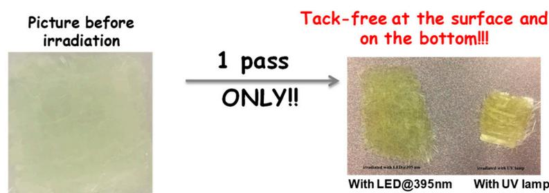
**Figure 13.** FRP experiments of a BisGMA/TEGDMA (70%/30%) blend for composites cured using an LED emitting at 395 nm. Reprinted/adapted with permission from Ref. [254]. Copyright 2018, The American Chemical Society.
