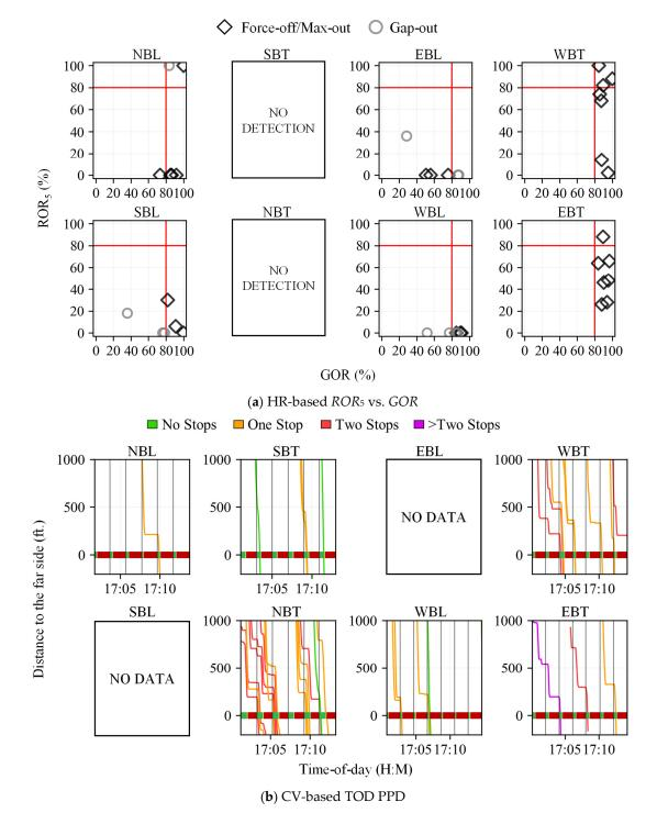
**Figure 3.** HR and CV split failure evaluation for relevant movements from 17:00 to 17:15 hrs. on 24 May 2023.
