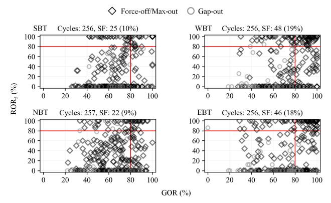
(a) HR-based ROR5 vs. GOR (Figure 7, callout ii) displaying the number of cycles that split failed (SF)
