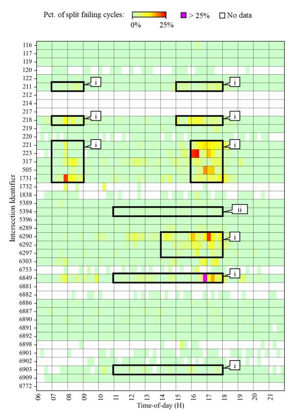
**Figure 8.** Percentage of through movement cycles with presence stop bar detection that split failed according to CV data from 06:00 to 22:00 hrs. from 22 May 2023 to 26 May 2023.
