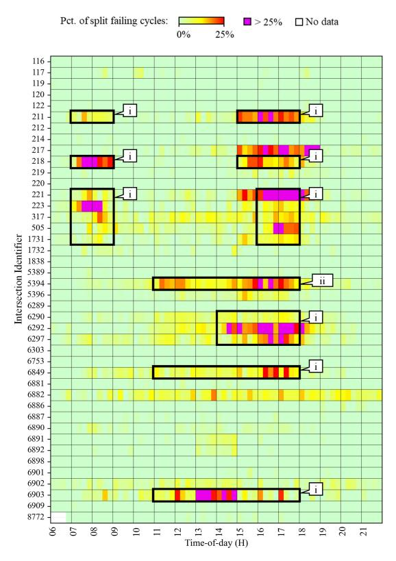
**Figure 7.** Percentage of through movement cycles with presence stop bar detection that split failed according to HR data from 06:00 to 22:00 hrs. from 22 May 2023 to 26 May 2023.
