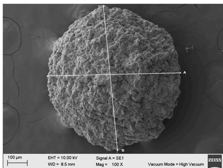
**Figure 1.** SEM micrograph of produced microcapsules. Segment A is 671.2  $\mu\text{m}$  long; segment B is 744.8  $\mu\text{m}$  long.
