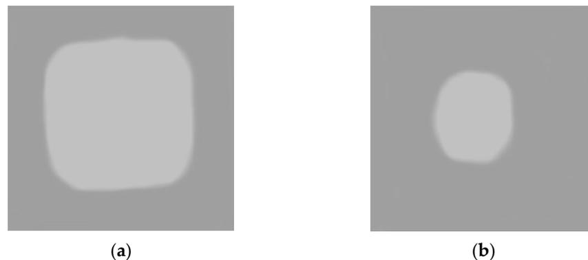
**Figure 7.** Thickness of the dark area of ceramic composite materials based on plasma-chemical powders based on  $\text{Si}_3\text{N}_4$ ,  $\text{Si}_3\text{N}_4\text{—TiN}$ , SIALON—TiN vs. dwell time of hot pressing: (a)—1 min, (b)—8 min.
