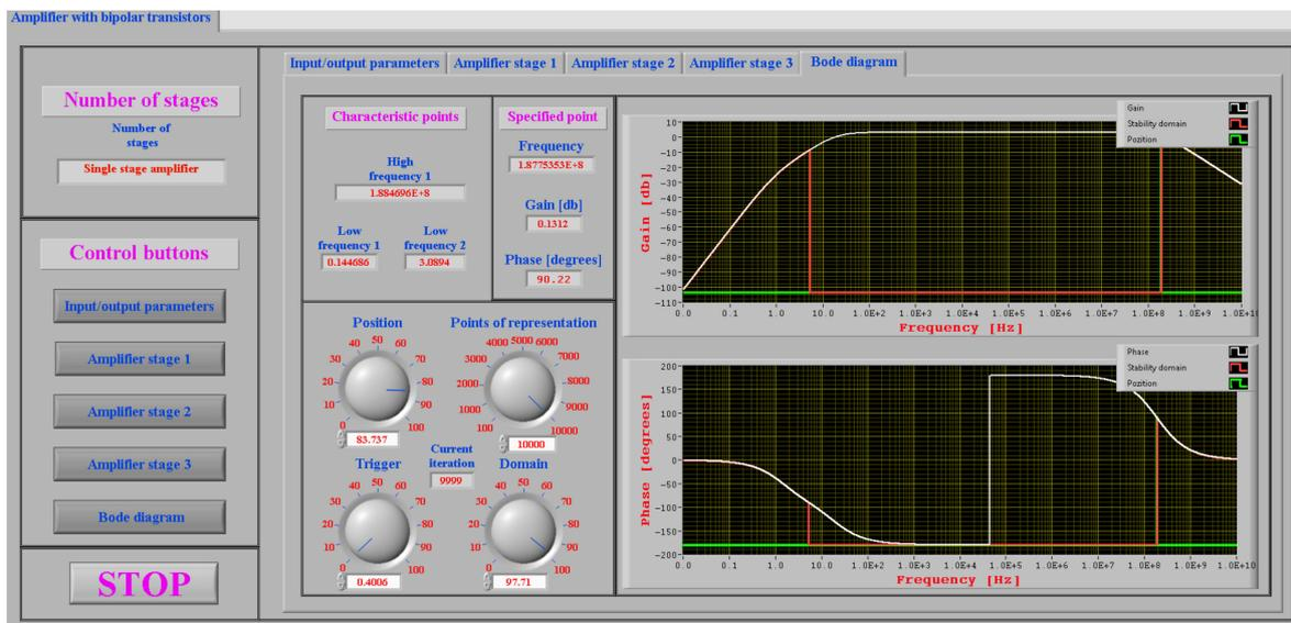
Figure 28. Bode diagram for line 4 from Table 1 with  $SW_{CEe1}$  to OFF, for high cut frequency of 188.7 MHz.
