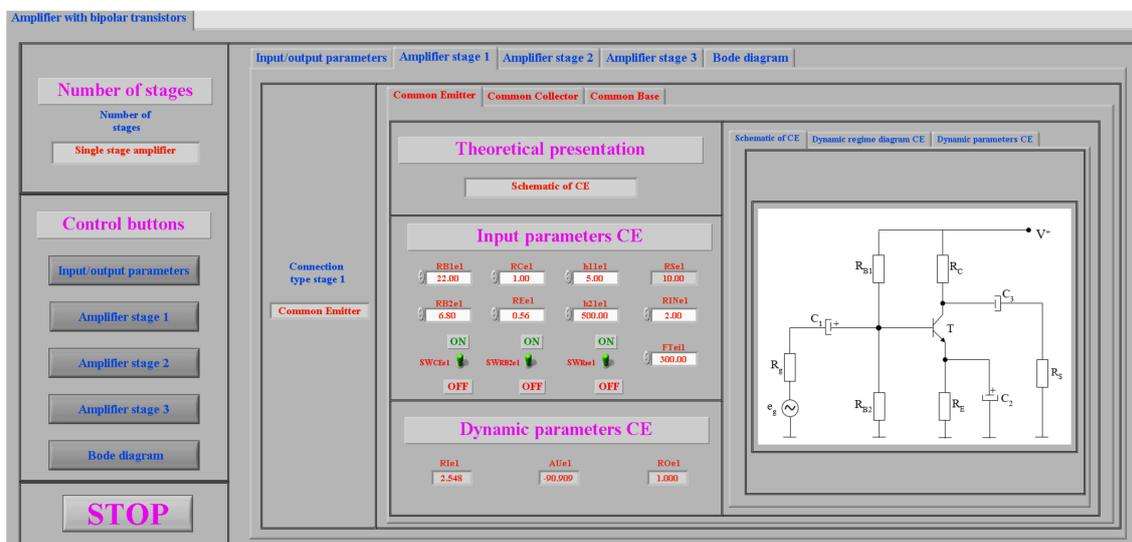
Figure 9. Front panel for common emitter stage parameters.
