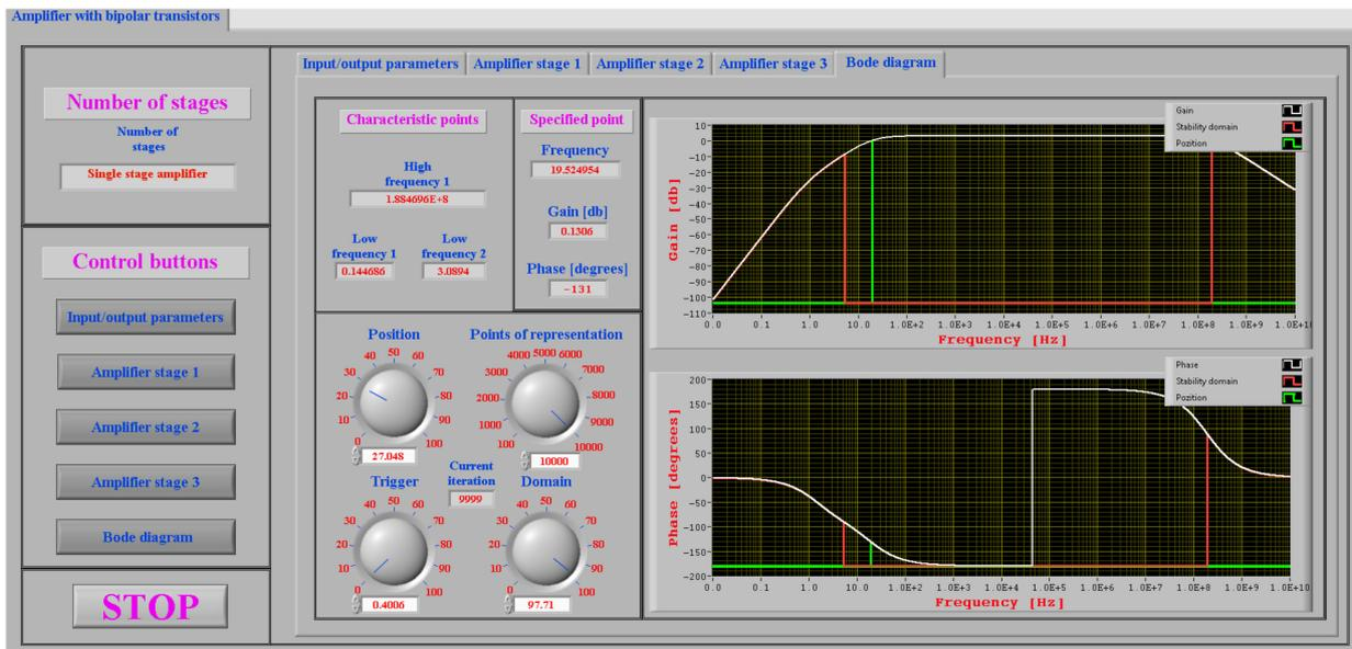
Figure 27. Bode diagram for line 4 from Table 1 with  $SW_{CEe1}$  to OFF, for low cut frequency of 19.5 Hz.
