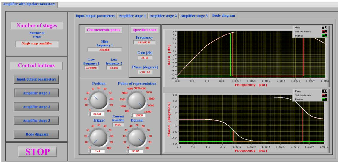
Figure 21. Bode diagram for line 8 from Table 1 with  $SW_{CEe1}$  to ON, for low cut frequency of 38.66 Hz.
