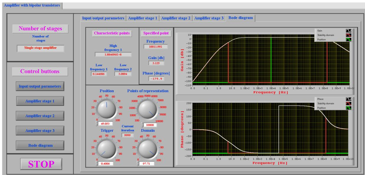
Figure 26. Bode diagram for line 4 from Table 1 with  $SW_{CEe1}$  to OFF, for 10 kHz frequency.
