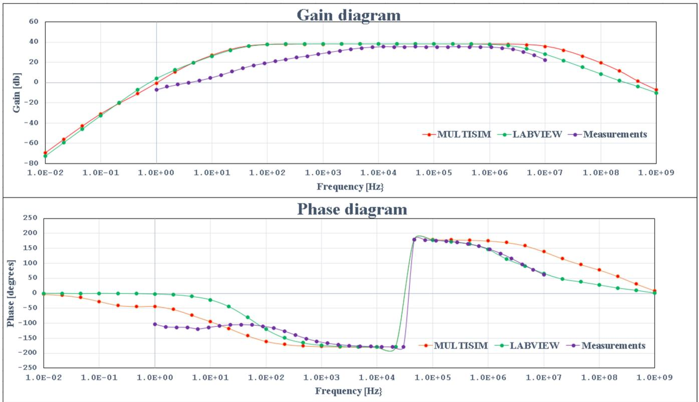
Figure 25. Simulations and experimental results for common emitter connection with  $SW_{CEe1}$  to ON.
