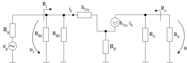
**Figure 3.** The equivalent scheme in dynamical regime for a common emitter connection.
