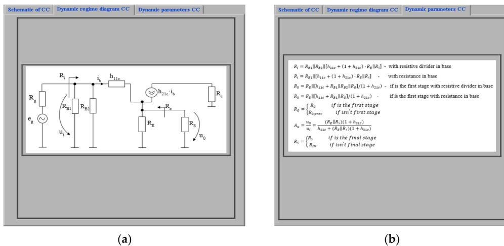
Figure 13. (a) Dynamic regime diagram CC, (b) Dynamic parameters CC.
