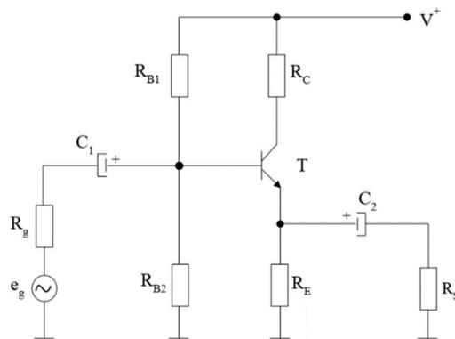
**Figure 4.** Electronic scheme for a common collector connection.
