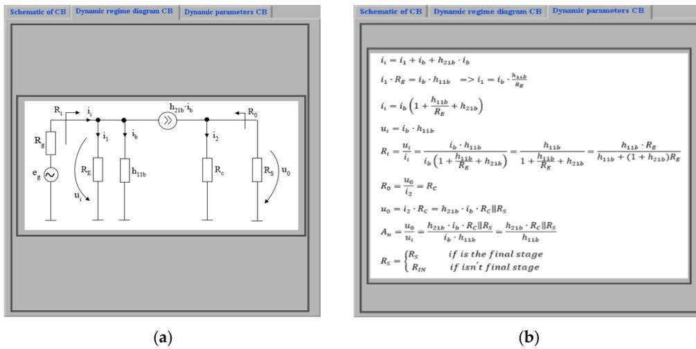
Figure 16. (a) Dynamic regime diagram CB, (b) Dynamic parameters CB.
