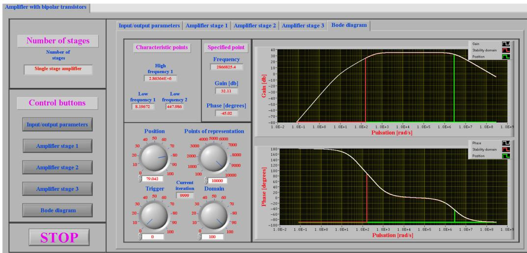
Figure 37. Bode diagram for line 1 from Table 3, for high cut pulsations of 2.86 MHz.
