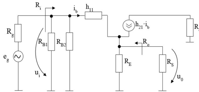
Figure 5. The equivalent scheme in dynamical regime for a common collector connection.
