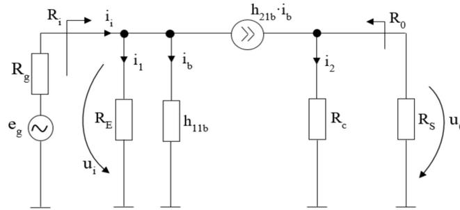
Figure 7. The equivalent scheme in dynamical regime for a common base connection.
