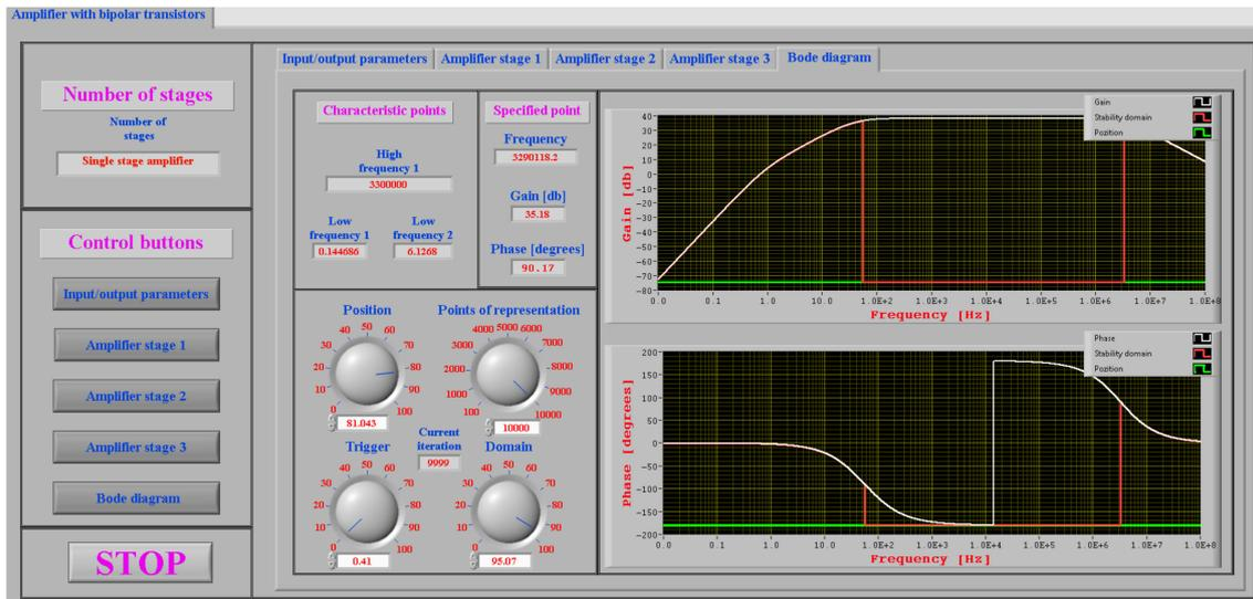
Figure 22. Bode diagram for line 8 from Table 1 with  $SW_{CEe1}$  to ON, for high cut frequency of 3.29 MHz.
