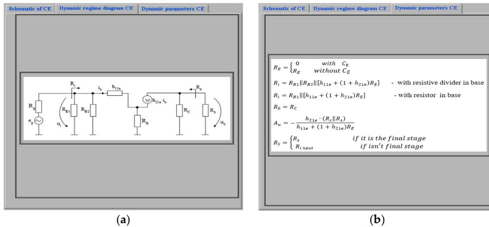
Figure 10. (a) Dynamic regime diagram CE, (b) Dynamic parameters CE.
