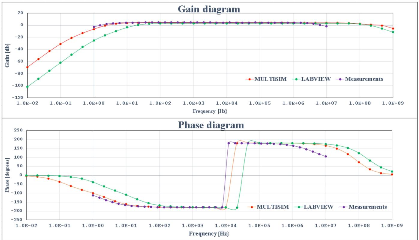
Figure 29. Simulations and experimental results for common emitter connection with  $SW_{CEe1}$  to OFF.
