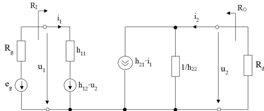
**Figure 1.** An equivalent circuit of an amplifier stage using the quadrupole “h” parameters.
