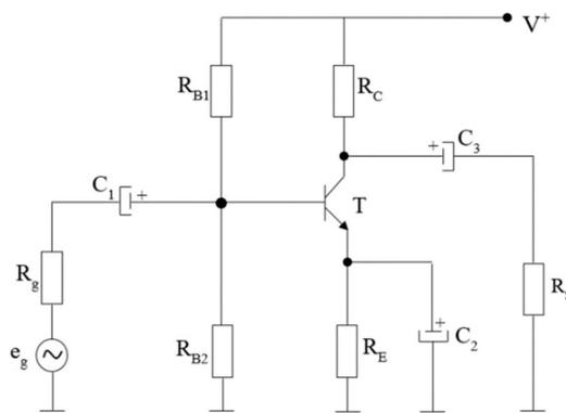
Figure 2. Electronic scheme for common emitter connection.
