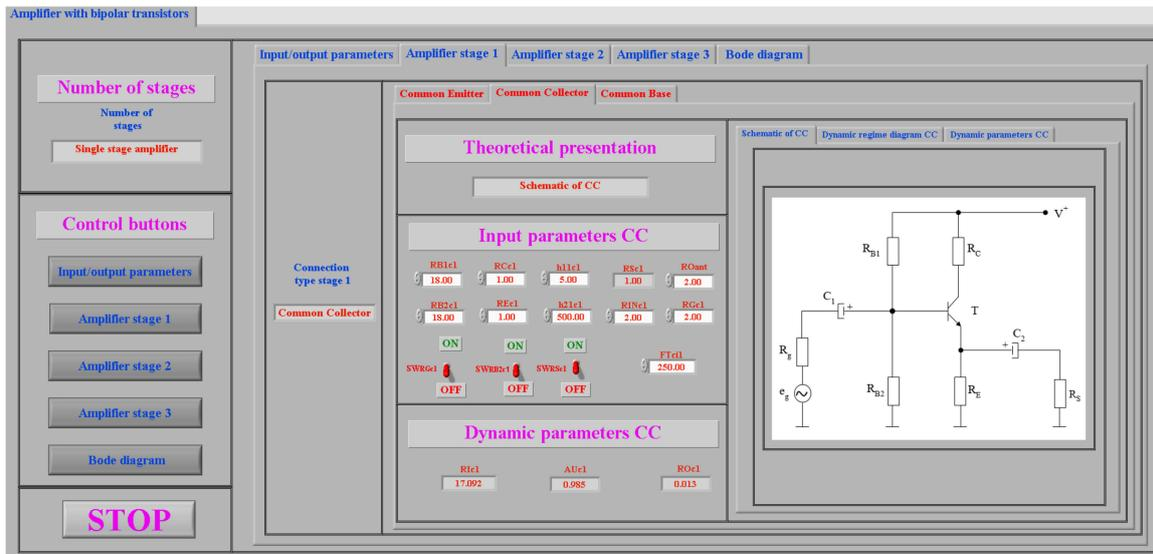
Figure 12. Front panel for common collector stage parameters.
