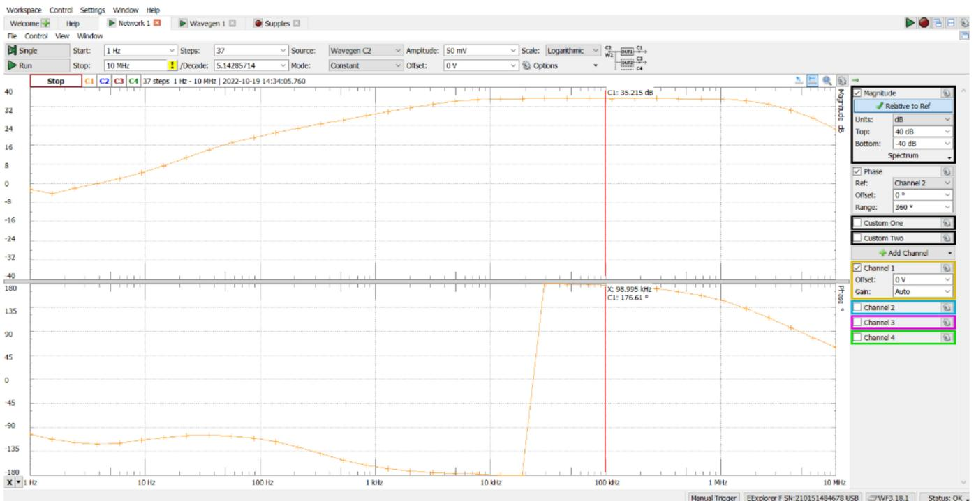
Figure 24. Measurement results for common emitter connection with  $SW_{CE1}$  to ON, using Electronic Explorer Board.
