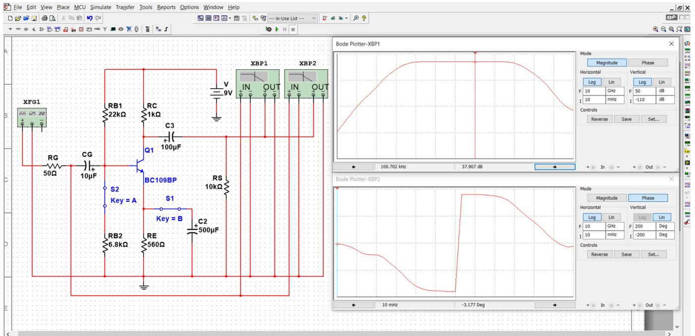
Figure 23. Simulation results for common emitter connection with  $SW_{CE1}$  to ON, using Multisim.
