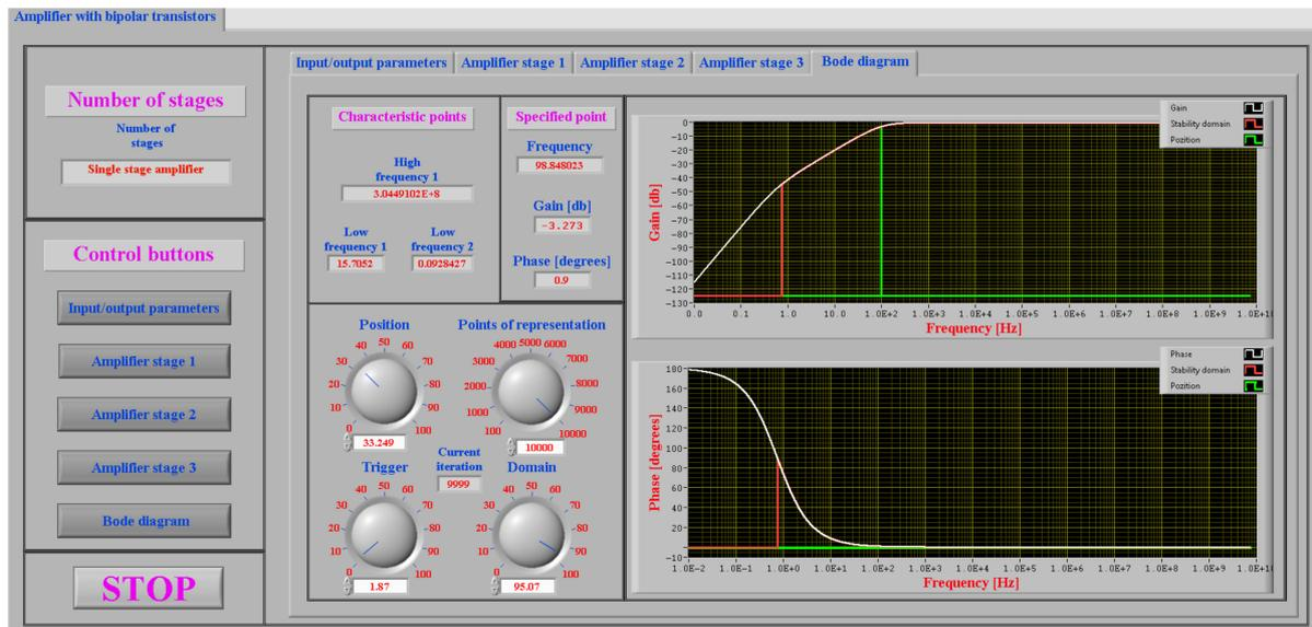
Figure 31. Bode diagram for line 5 from Table 2, for low cut pulsations of 98.85 Hz.
