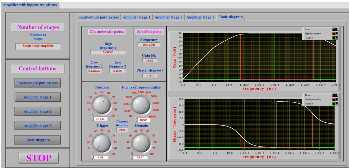
**Figure 20.** Bode diagram for line 8 from Table 1 with SW<sub>CEe1</sub> to ON, for 10 kHz frequency.
