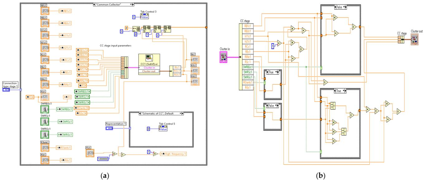
Figure 14. (a) Program implementation of computed parameters, (b) Subroutine CC1.
