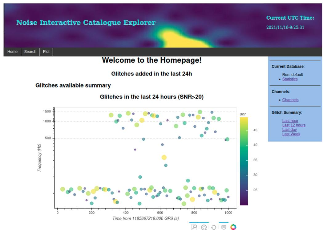
**Figure 2.** The NICE Homepage—Visualizing simulated glitches. The scatter plot in the center reports the metadata corresponding to peak time (x-axis), and central frequency (y-axis, logarithmic scale) of triggers in the time interval of ~18 min from 00:00 of 2 August 2017. If the collaboration is acquiring data, this page shows real Virgo glitches collected during the last 24 h.
